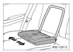
3 Shake the ISOFIX platform (1) strongly to check that it is firmly attached.
