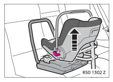
2 Lift the baby carrier (14) to check that it has been correctly and securely attached to the base frame (8).
