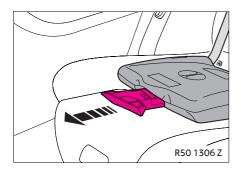
4 Press the locking button below the locking arm release handle (7) and pull the release handle out on the front end of the ISOFIX platform (1).
