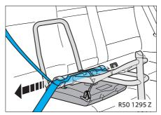
10 Put the shoulder belt into the belt guide (9) in parallel to the lap belt and pull the shoulder belt tight as well.
