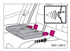
You will hear an audible locking sound. The ISOFIX platform (1) is firmly connected to the car and it is no longer loose.
