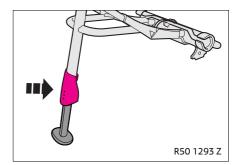
The support leg (12) moves down and presses against the floor of the car.
