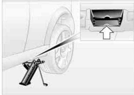
2. During jacking up, insert the jack head in the square recess of the jacking point
