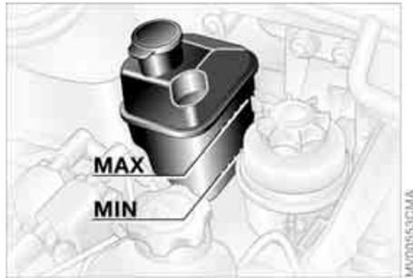
As an example, the illustration shows the coolant tank of the MINI COOPER and the MINI COOPER Convertible.
