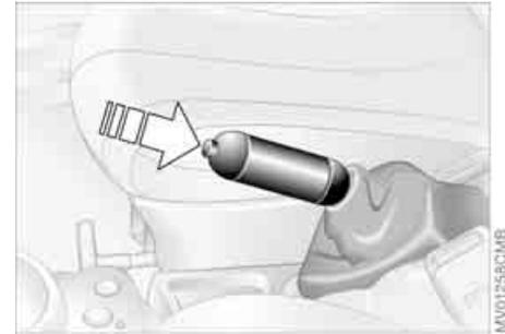
The parking brake is designed primarily to prevent the vehicle from rolling when it is parked. It operates against the rear wheels.
