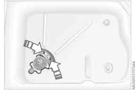
5. Squeeze the securing spring
