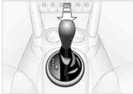
▶ If the engine speed is too high when the vehicle is at a standstill, the selector lever is also blocked to protect the transmission.
