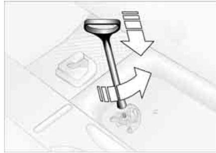
3. Screw the lifting handle from the onboard tool kit onto the thread
