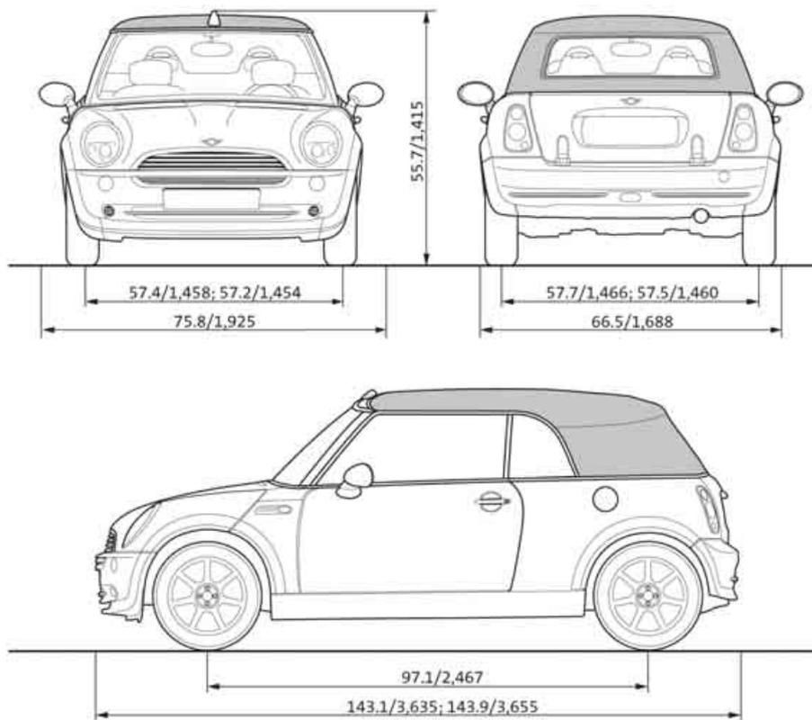
All measurements in inches/millimeters. Smallest turning circle dia. 34 ft 10 in/10.66 m.
