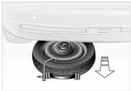
9. Pull out the space-saver spare tire towards the rear underneath the vehicle
