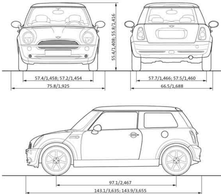
All measurements in inches/millimeters. Smallest turning circle dia. 34 ft 10 in/10.66 m.
