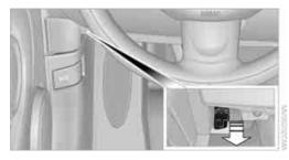
Primary components that make up exhaust emissions can be checked by a device via the OBD socket.
