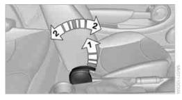
Pull the lever, arrow 1, and apply your weight to the backrest or lift it off, as necessary, arrows 2.
