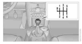
When shifting into 5th or 6th gear, press the gearshift lever to the right. Otherwise the engine could be damaged if you inadvertently shift into 3rd or 4th gear. ◀
