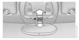
To switch the interior lamps on/off.
