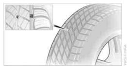
Wear indicators in the base of the tread groove are distributed around the tire's circumference; the letters TWI, for Tread Wear Indicator, on the tire's sidewalls identify tires that incorporate these wear indicators. When tire tread is worn down to the level of the wear indicators, the remaining tread depth is 1/16 in/1.6 mm.
