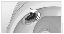
4. Screw out the bulb counterclockwise.
