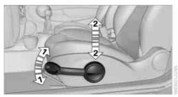
Pull up or push down the lever repeatedly, arrows 1, until the desired height is reached, arrows 2.
