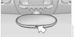
The automatic dimming feature of the interior rearview mirror\* is controlled by two photo cells in the mirror. One photo cell is in the mirror frame, arrow; the other is on the back of the mirror.
