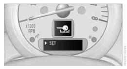
Press and hold the button until the display changes. Briefly press the button repeatedly until "RESET" is displayed.
