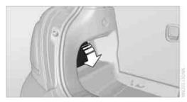
2. Pull on the green knob with the fuel pump symbol. The fuel filler door is released.
