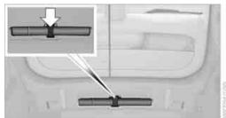
In the cargo bay under the loading sill. Open the center lock to take it out.
