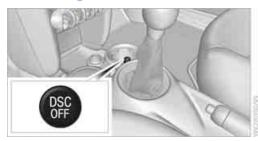
Press the button repeatedly until the DSC indicator lamps come on. DSC is deactivated. Stabilizing and propulsion promoting actions are no longer executed.
