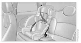
All rear safety belts and the safety belt for the front passenger can be prevented from being pulled out in order to secure child-restraint systems.
