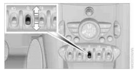
The switch locks or unlocks the doors and tailgate when the doors are closed, but the antitheft system is not activated. The fuel filler door remains unlocked\*
