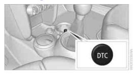
Press the button for at least 3 seconds: the DSC indicator lamps come on. The dynamic traction control (DTC) and dynamic stability control (DSC) are both deactivated. There will be no more stabilizing interventions.
