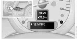
Press and hold the button until the display changes. 4. Briefly press the button repeatedly until the symbol and "SET" are displayed.
