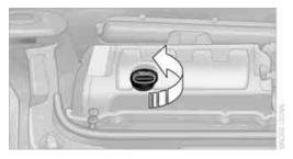
Do not add the maximum quantity of 1 US guart/1 liter of engine oil until the oil level has dropped to just above the lower mark on the dipstick, page 104.
