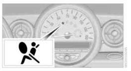
As of radio readiness, page 37, the warning lamp comes on briefly to indicate that the entire airbag system and the belt tensioners are operational.
