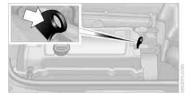
Attach the second terminal clamp of the minus/- jumper cable to the negative terminal of the battery or to the engine or body ground of the vehicle to be started.
