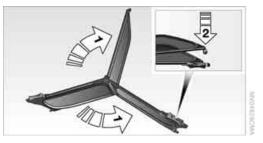
3. Press the locking device together until it engages, see arrow 2.
