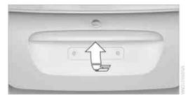
Press the button in the handle, arrow, or the button of the remote control, for an extended period. The liftgate is unlocked and can be opened.
