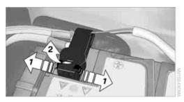
Attach one terminal clamp of the plus/+ jumper cable to the positive terminal of the battery or to a starting-aid terminal of the vehicle providing assistance.
