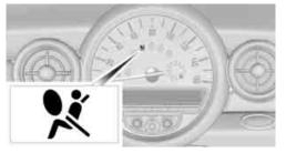
As of radio readiness, page 44, the warning lamp comes on briefly to indicate that the entire airbag system and the belt tensioners are operational.
