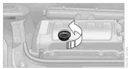
Do not add the maximum quantity of 1 US guart/1 liter of engine oil until the oil level has dropped to just above the lower mark on the dipstick, page 128.
