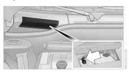
2. Release the tabs on the left and right sides of the positive terminal cover\*, arrows 1, and lift the cover to open, arrow 2.
