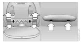
To switch the reading lamps on and off. In front: press the switch. In the rear: press the button.
