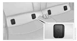
The anchor points for the lower LATCH anchors are located behind the labeled protective caps.
