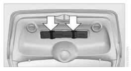
On the inside of the liftgate. Press the tab to take it out.
