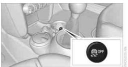
Press the button repeatedly until the DSC indicator lamps come on. DSC is deactivated. Stabilizing and propulsion promoting actions are no longer executed.
