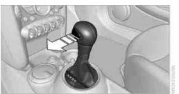
Move the selector lever from position D to the left into the M/S shifting slot:
