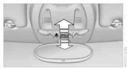
To switch the interior lamps on/off.
