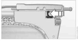
Push the release lever toward the center of the wind deflector and fold both halves together.
