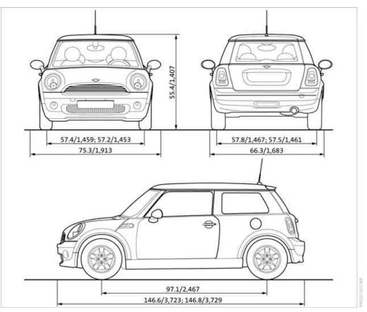
All dimensions in inches/mm. Minimum turning radius  $\emptyset$ : 35 ft 10 in/10.7 m. Information after the semicolon: different values for MINI Cooper S.
