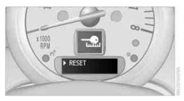
Press and hold the button until the display changes to the first setting. The settings are reset.
