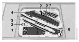
On vehicles with a space-saver spare tire, the tire change set with onboard tools is stored under the floor mat in the cargo area.
