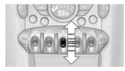
The switch locks or unlocks the doors and liftgate when the doors are closed, but the antitheft system is not activated. The fuel filler flap remains unlocked\*.
