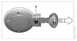
Press button 1 to release the key. The integrated key fits the following locks:
