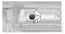
Do not add the maximum quantity of 1 US guart/1 liter of engine oil until the oil level
