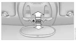
To switch the interior lamps on/off. Press the switch.
