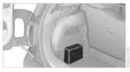
The first aid pouch is located on the rear cargo well by the left side trim panel or under the flat load floor.
