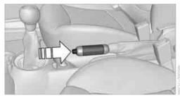
Pull slightly upward, press the button and lower the lever.
