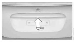
Press the button in the handle, arrow, or the button of the remote control, for an extended period. The tailgate is unlocked and can be opened.
