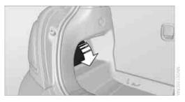
2. Unscrew the desired bulb counterclockwise, arrows **1**.
