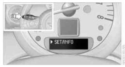
Press and hold the button until the display changes. Press the button repeatedly until the corresponding symbol and "CHECK INFO" appear in the display.
