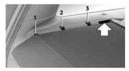
The roll-up cover can be removed to load bulky luggage.
