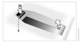
Insert the snap-in adapter at the front, arrow 1, and press downward, arrow 2, until it clicks into place.
