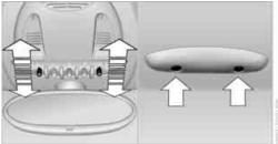
To switch the reading lamps on and off In the front: press the switch. In the rear: press the button.
