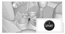
Press the button. The LED lights up. SPORT is briefly displayed in the tachometer.
