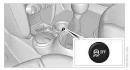
Press the button until the DSC OFF indicator lamp on the speedometer is on and DSC OFF is displayed on the tachometer. DSC is deactivated. Stabilizing and propulsion promoting actions are no longer executed.
