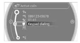
Enter the DTMF code via the onboard computer.
