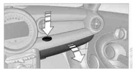
Press the button to open the cover. The light in the glove compartment comes on.
