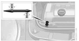
The oil quantity corresponding to the difference between the two marks on the dipstick is 1 US guart/1 liter.
