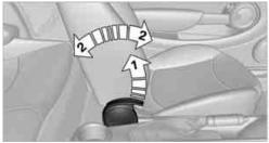
Pull the lever, arrow 1, and apply your weight to the backrest or lift it off, as necessary, arrows 2.
