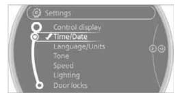
4. Turn the MINI joystick until "Time:" is selected, and press the MINI joystick.
