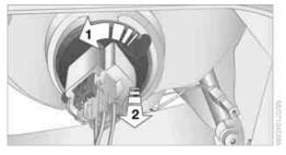
2. Push on the catch, arrow **1**, and disconnect the connector, arrow **2**.
