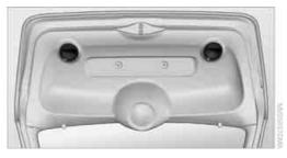
The handle recesses on the interior trim panel of the tailgate make it easier to pull it down.
