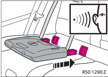
You will hear an audible locking sound. The ISOFIX platform (1) is firmly connected to the car and it is no longer loose.
