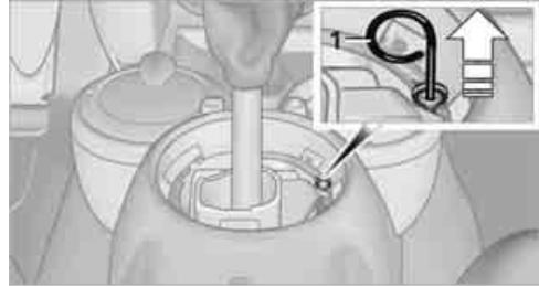
3. Take the hub cover remover 1 out of the onboard tool kit and insert it in the loop on the front passenger side.
