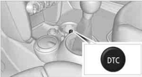
Press the button: the DTC indicator lamps come on.
