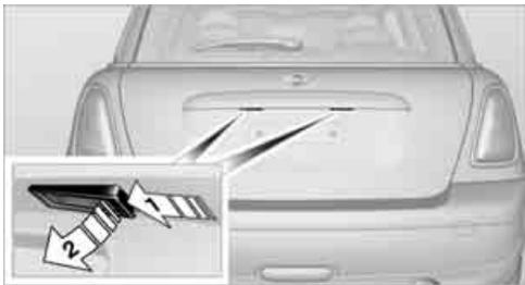
1. Using a screwdriver, push the lamp to the left in the tab of the lamp housing, arrow 1.
