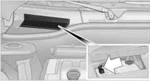
2. Attach one terminal clamp of the plus/+ jumper cable to the positive terminal of the battery or to a starting-aid terminal of the vehicle providing assistance.
