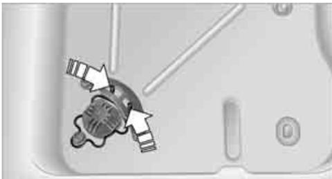
6. The space-saver spare tire is released and must be held by the lifting handle.
