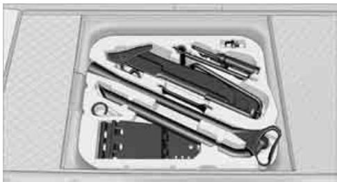
Your vehicle comes with an onboard tool kit that varies with the equipment version; it is stored underneath the level load floor.
