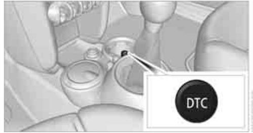
Press the button for at least 3 seconds: the DSC indicator lamps come on. The dynamic traction control (DTC) and dynamic stability control (DSC) are both deactivated. There will be no more stabilizing interventions.
