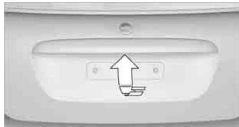
Press the button in the handle, arrow, or the
