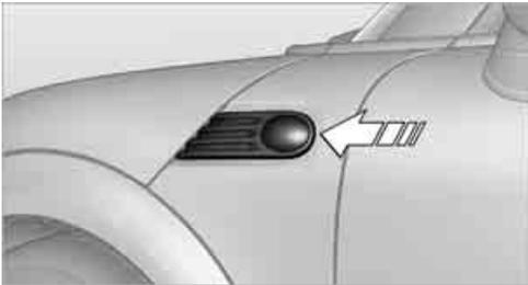
2. Screw out the bulb holder counterclockwise.
