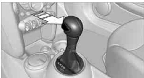
Press the button on the front of the selector lever, arrow.
