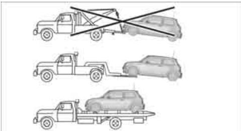
Have the MINI transported with a tow truck with a so-called lift bar or on a flat bed.
