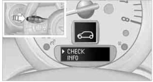
4. Hold the button down. "CHECK OK" appears if there are no Check Control messages. If a Check Control message has been stored, the corresponding message is displayed.
