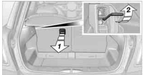
1. Pull the lever, arrow 1, and fold the rear seat backrest forward.
