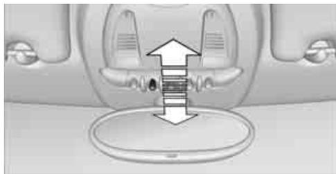
To switch the interior lamps on/off.
