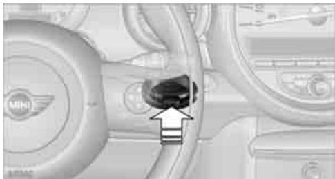
Insert the key all the way into the ignition lock.
