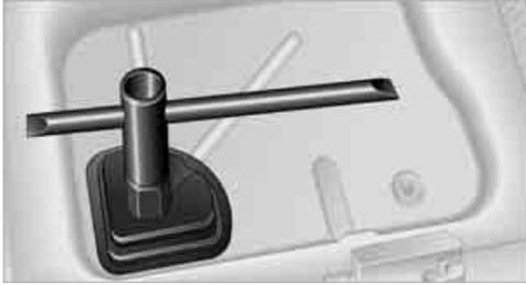
3. Screw the lifting handle from the onboard tool kit onto the thread.
