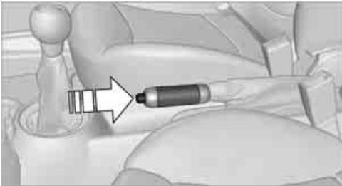
Pull slightly upwards, press the button and lower the lever.
