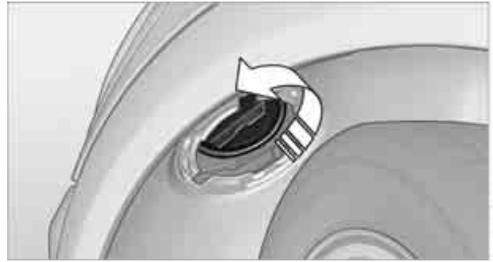
3. To insert the new bulb and replace the cover, proceed in reverse order.
