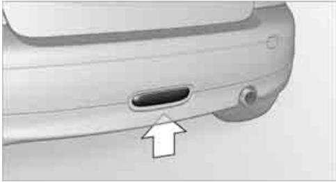
1. Screw out the bulb holder counterclockwise.
