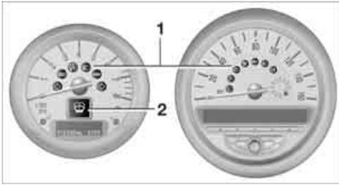
Indicator and warning lamps can light up in various combinations and colors in indicator area 1 or 2. See the table for information on causes and how to react. Note whether a lamp comes on alone or in combination with another. Some lamps can light up in different colors. Corresponding distinctions are made in the text.
