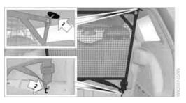
Insert each partition net mounting pin all the way into its respective rear mount in the headliner, arrow 1, and push it forward.
