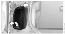
Swing out the tail lamp and remove it toward the top. 3. Disconnect the cable connector if necessary, arrow 1.
