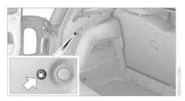
Pull on the green knob with the fuel pump symbol; the fuel filler flap opens.
