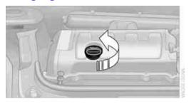
Do not add the maximum quantity of 1 US guart/1 liter of engine oil until the oil level has dropped to just above the lower mark on the dipstick, page 118.
