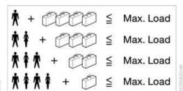
The permissible load is the sum of the occupants' weights and the weight of the cargo. The greater the weight of the occupants, the less cargo/luggage can be transported.
