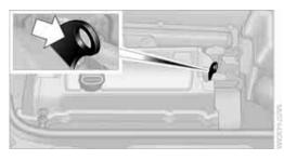
Attach the second terminal clamp of the minus/- jumper cable to the negative terminal of the battery or to the engine or body ground of the vehicle to be started.
