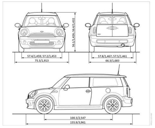
All dimensions in inches/mm. Minimum turning radius  $\emptyset$ : 36 ft in/11.0 m. Information after the semicolon: different values for MINI Cooper S.
