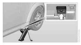
2. During jacking up, insert the jack head in the square recess of the jacking point.
