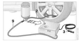
Unscrew the dust cap from the valve of the defective wheel and screw the filling hose 2 of the sealant bottle onto the valve.
