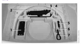
In vehicles with the space-saver spare tire, the tire change set with the onboard vehicle tool kit is located beneath the floor mat or flat load floor in the cargo area.
